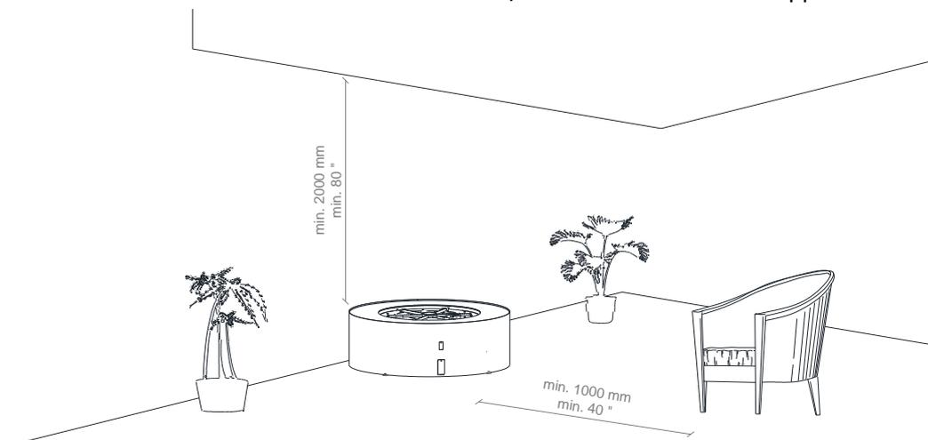
Fig. 1: Minimum distance to flammable materials
