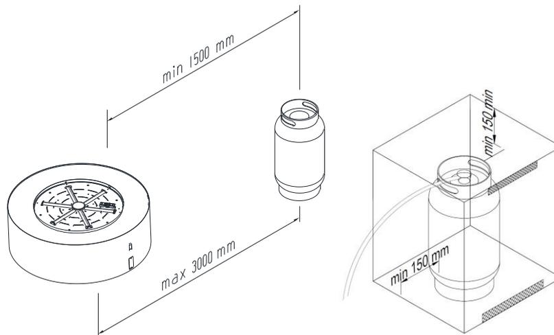
Fig. 4 – Gas cylinder distnace
