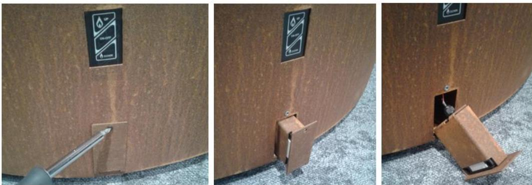
*Fig. 8: Removing of the battery container*
