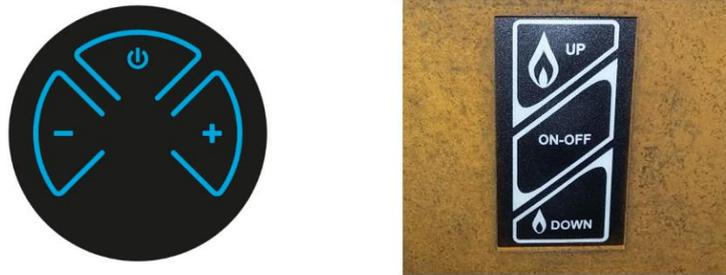
Fig. 5: Hand-held transmitter and Touch Panel
