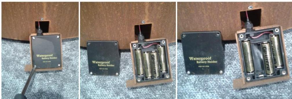
*Fig. 9: Replacing the batteries in the container*
