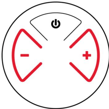
Pressing the „+“ button twice automatically increases the flames to the HIGH position
